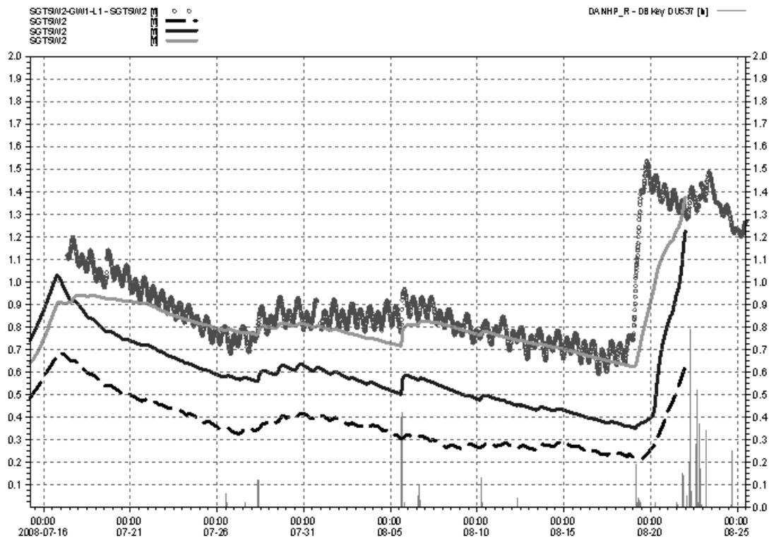
Figure 7: The observed groundwater (symbols), local rainfall (bars) and simulated groundwater levels using different groundwater models prior to and during the tropical storm Fay
