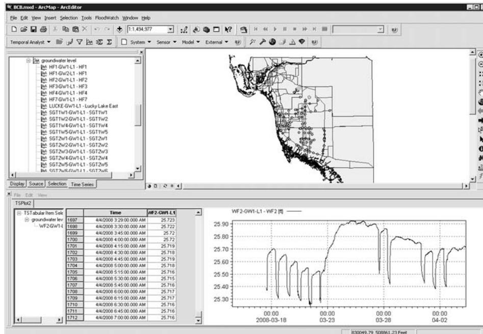
**Figure 3: Examples of the GIS interface showing spatial data, plots and tabulations for a groundwater monitoring point**
