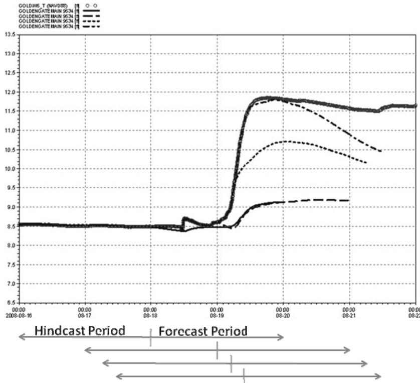
Figure 6: The observed water levels (symbols) and forecasted water levels (lines) for the sequence of 4 forecasts used to evaluate the model during tropical storm Fay
